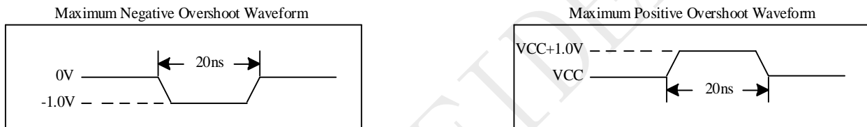
Figure 5-2 Input Test Waveforms and Measurement Level
